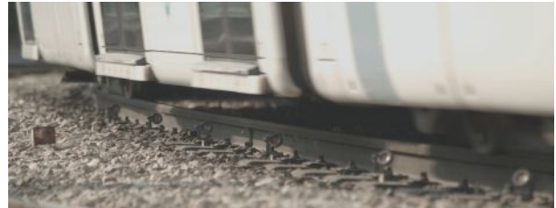
PRISMS AFFIXED TO THE TRACK enable measurement of change and structural movement.
